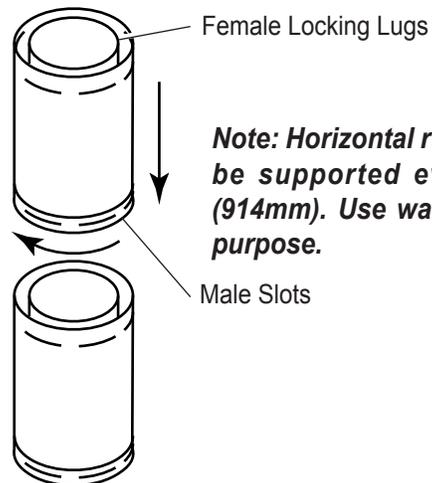
**Note: Horizontal runs of vent must be supported every three feet (914mm). Use wall straps for this purpose.**
