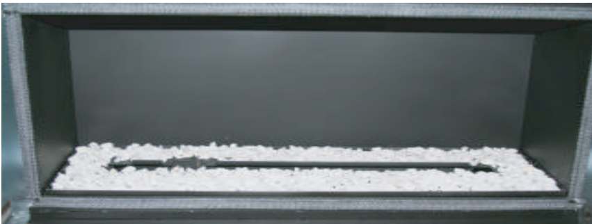
Figure 39 - Filling the tray with media
