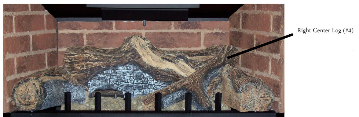
Figure 20 - Installing Right Center Log #4
