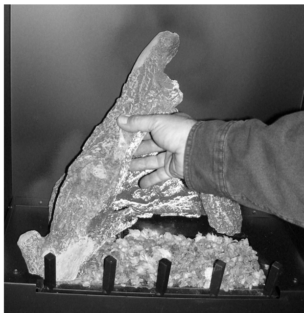
Figure 39 - Placing Front Left Log (#2)
