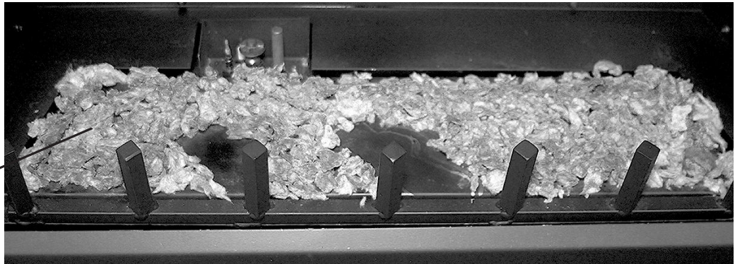
Figure 16 - Rock Wool Placement
